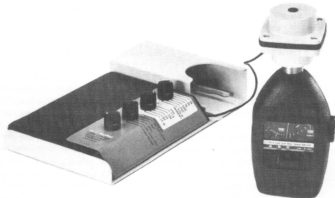
Figure 2-3. Typical calibration setup with a GR 1565-B Sound-Level Meter.
