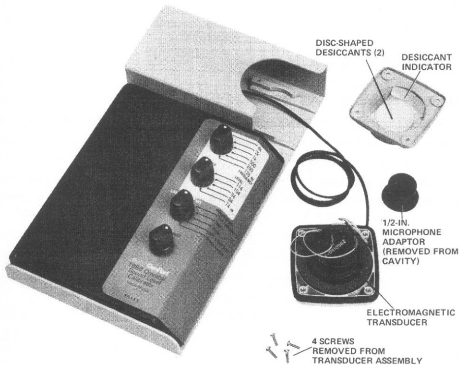
Figure 2-2. Transducer assembly disassembled.
